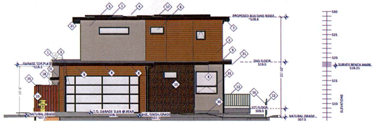
2 FRONT ELEVATION (NE) scale 1/4" = 1'-0"
